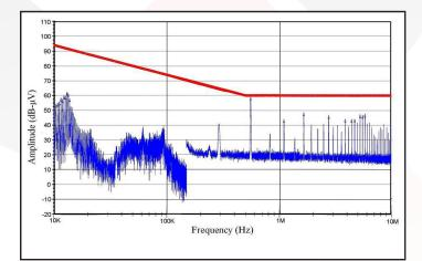
Figure 22: High frequency conducted emissions of standalone MQHL-28-05S, 5Vout module at 50W output, as measured with Method CE102. Limit line shown is the 'Basic Curve' for all applications with a 28V source.
