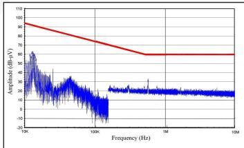
Figure 23: High frequency conducted emissions of MQHL-28-05S, 5Vout module at 50W output with MQHE-28-P filter, as measured with Method CE102. Limit line shown is the 'Basic Curve' for all applications with a 28V source.
