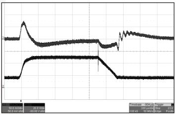
**Figure 12**: Output voltage response to step-change in input voltage (16V - 50V - 16V) in 150µS. Ch 1: Vout (50mV/div). Ch 2: Vin (20V/div).
