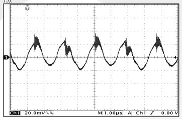
**Figure 15**: Output voltage ripple, Vout, at nominal input voltage and rated load current (20mV/div). Load capacitance:  $1\mu F$  ceramic capacitor and  $10\mu F$  tantalum capacitor. Bandwidth: 10MHz. See Figure 13.
