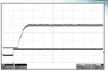
*Figure 8*: Turn-on transient at full resistive load and 5mF output capacitance initiated by ENA1. Input voltage pre-applied. Ch 1: Vout (500mV/div). Ch 3: ENA1 (5V/div).
