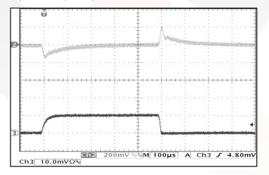
**Figure 11**: Output voltage response to step-change in load current 0%-50%-0% of lout (max). Load cap:  $1\mu$ F ceramic cap and  $10\mu$ F,  $100m\Omega$  ESR tantalum cap. Ch 1: Vout (200mV/div). Ch 2: lout (10A/div).
