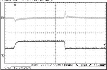
**Figure 10**: Output voltage response to step-change in load current 50%-100%-50% of Iout (max). Load cap:  $1\mu$ F ceramic cap and  $10\mu$ F,  $100m\Omega$  ESR tantalum cap. Ch 1: Vout (200mV/div). Ch 2: Iout (10A/div).
