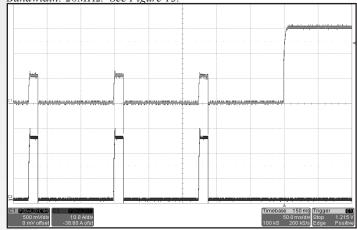
*Figure 16*: *Rise of output voltage after the removal of a short circuit across the output terminals. Ch 1: Vout (500mV/div). Ch 2: Iout (10A/div).*
