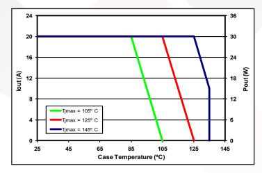
**Figure 5**: Output Current / Output Power derating curve as a function of Tcase and the Maximum desired power MOSFET junction temperature at Vin = 28V (see Note 12).
